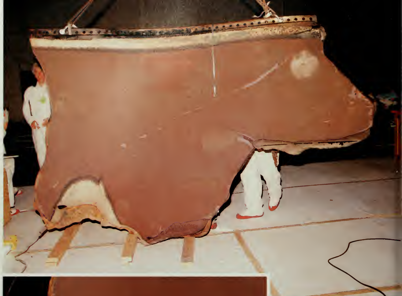
At upper left is the aft segment burn viewed from inside the casing; the lower photo is a closeup of the same section. The latter photo shows a hole (arrow) where the flame plume may have burned through the casing from the outside. At right is a composite view of the burn above and below the aft field joint.
